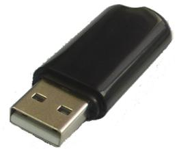
The MEGAPOWER M-Pointer uses state-of-the-art image processing technology to capture and trace the movement of IR light on the pen. All PC mouse function are fully supported. It expands existing projector installation to Interactive capability. Lectures can be delivered interactively and notes recorded and stored in computer. For bussiness presentations, the portability of this M-Pointer makes it easy to deliver interactive presentations on the go, creating more attention from audience.
